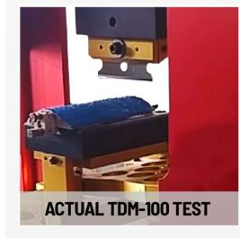
BLADE IS MOVED 20 MM ACROSS TEST MATERIAL
